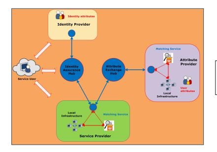
High-level technical architecture selected for Alpha project Much care was taken by the project team to design the attribute exchange system in such a way that it forms the basis of a platform that can be developed and enhanced to include future requirements as envisaged by the project team. These were derived from the design principles, future potential needs, privacy guidance and potential technical constraints, as part of the design process.
