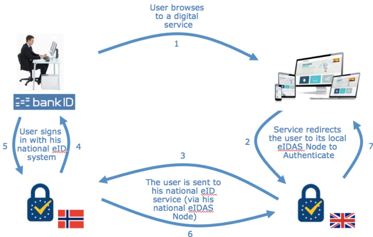
Figure 3 eID authentication under eIDAS - user accessing a UK service with a foreign (in this instance Norwegian) eID
